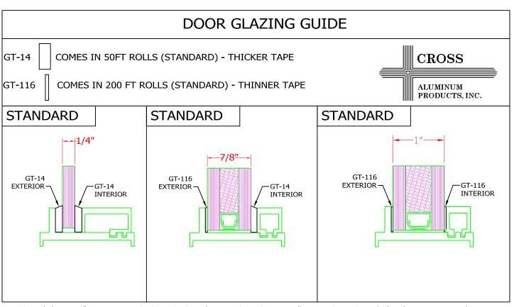
For additional glazing infill requirements, check out the door glazing guide inside our installation guide. Guide available online at www.crossaluminum.com.
